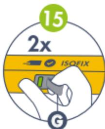
**15** Open the ISOFIX connectors (**F**) by pulling on the ISOFIX release puller (**G**) right on the side of the connectors.
