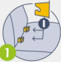
**1** If needed, place the two ISOFIX guides (**I**) on both ISOFIX anchor points between the seat and the backrest.
