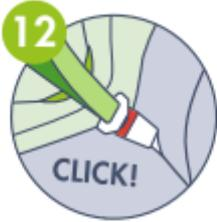
**12** Pull out the three-point belt, position it in front of the child and lock the belt tongue into the buckle of the vehicle.
