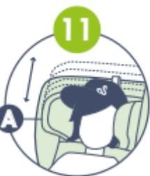
**11** Move the headrest (A) then slide it upward or downward. Adjust the headrest until the eye indicator matches the eye level of your child or you cannot put about two fingers (approximately 2 cm) between the shoulder of your child and the lower edge of the headrest.
