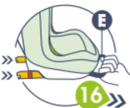
**16** Push the ISOFIX connectors back into the seat while pulling on the strap on the front (**E**) and then remove the seat from the vehicle.
