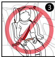
**! DO NOT allow the child to slouch, slide down in the seat, or create slack in the belt system 5. If child will not keep vehicle belt properly positioned, DO NOT use this booster seat.**
